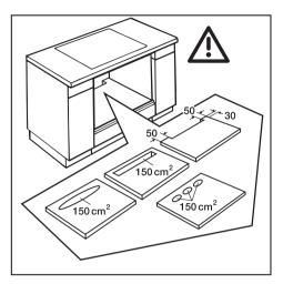
If an interim shelf is fitted beneath the oven, a cut-out is required as close to the unit back wall / the wall as possible to ensure that there is sufficient ventilation for the appliance.
